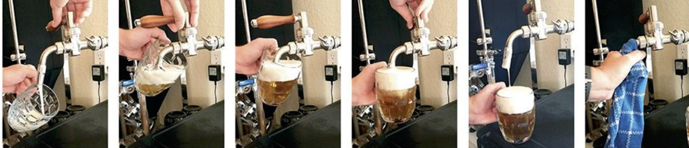
A Czech side-pull faucet can deliver just the right foam-liquid ratio to suit your personal tastes (and those of your guests).
